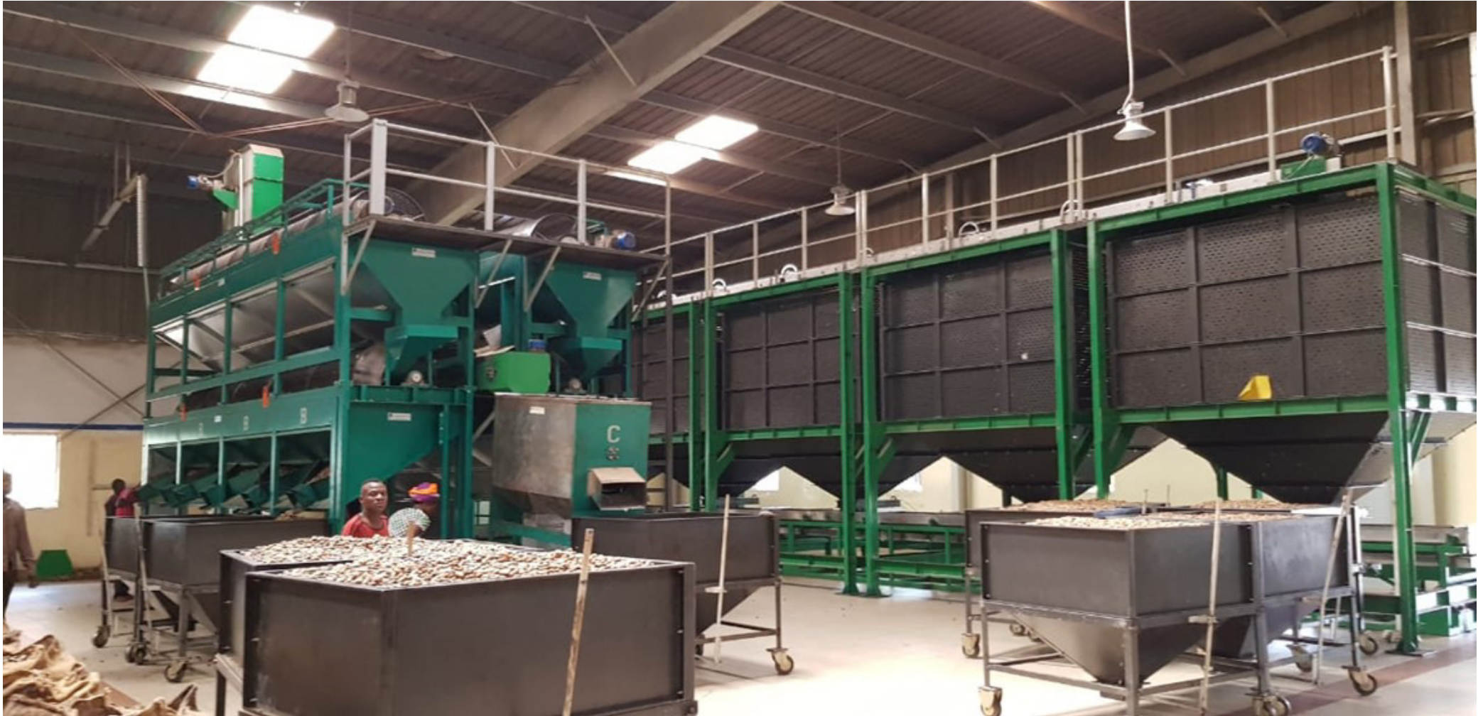
Post Cooking- RCN Auto Drying & Sizing Synchronisation
