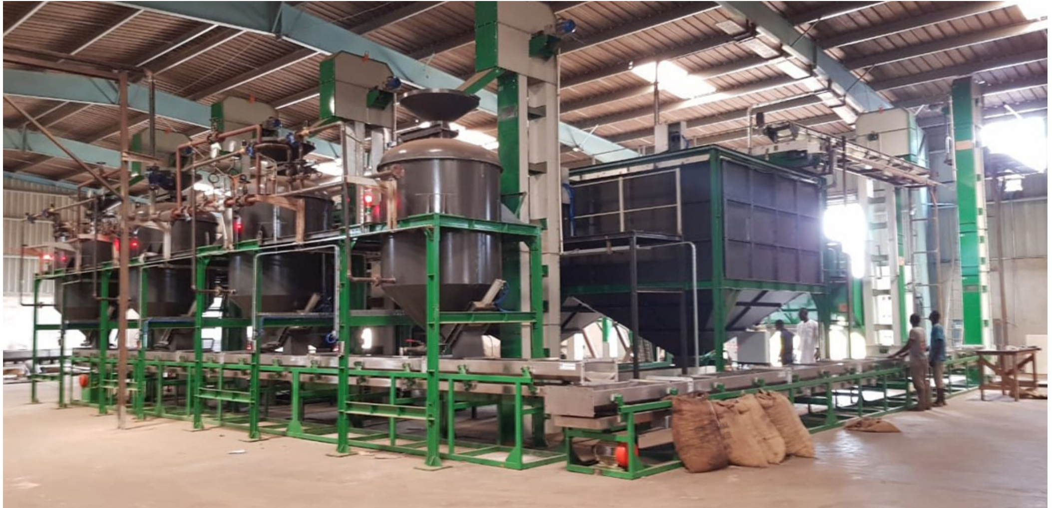
RCN Cleaning-Holding-Cooking- Transfer Synchronisation
